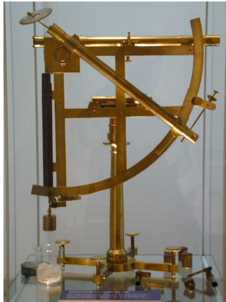
Fig 3. A Quadrant of 12 inches radius by John Bird, made in 1768 for the Royal Society's Transit of Venus Observations the following year. ( courtesy of the Royal Society )
